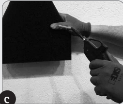
Blow the filter with an air gun
